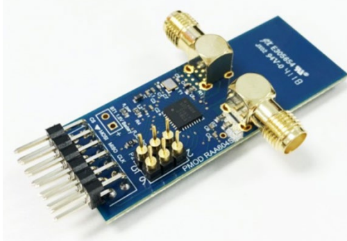
RAA604S002 WI-SUN TRANSCEIVER CHIP ON A "PMOD" EVALUATION MODULE.
